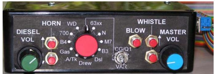
The remote control can have as many or as few of the above additional controls as required. They are all wired through to the remote control box via a 25-way ribbon cable, and can be connected to other external switches (eg reed switches or other sensors) if desired.
